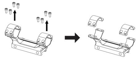
Figure 2-5 Unscrew the Ring Top
