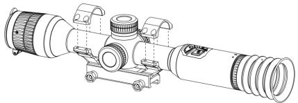
Figure 2-6 Put the Device in the Ring
