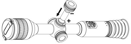
Figure 2-3 Install the Battery
