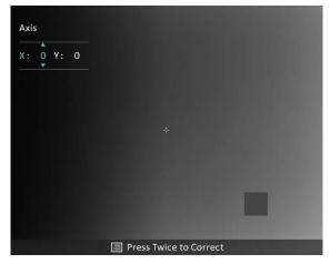
**Figure 3-5 Correct Defective Pixel**
