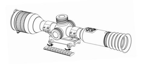
Figure 2-8 Loosen the Screws
